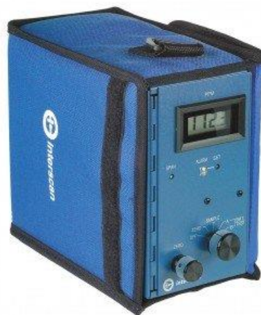
Figure 8. The Interscan 4160-1999b Portable Formaldehyde Gas Detector. It has a 0-1999 ppb range with a 0.2 ppb resolution.
