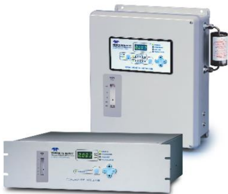
Figure 7. The Teledyne Model 465L UV Photometric Ozone Monitor. This Ozone monitor can detect ozone levels as low as 0 ppb and up to 500 ppm while sampling at 0.8 L/min
