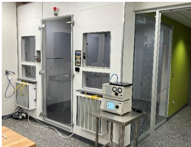
Figure 2: The 30 m 3 bioaerosol testing chamber at ARE Labs adheres to AHAM AC-5 standards and ASHRAE 241 criteria. The chamber is equipped with HEPA filtered air in/out, multiple bio aerosol sampling ports, decontamination, and pressure balance.
