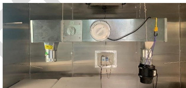
Figure 2: CASPR Medik X – Installed in partial HVAC duct used for testing in the bioaerosol test chamber.
