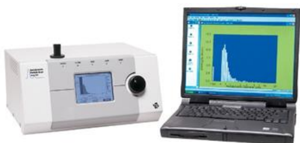
Figure 4. TSI Aerodynamic Particle Sizer (APS) model 3321 was used to measure the challenge bioaerosol's total particle concentration and particle size distribution. It has a 0.54-20.0 \mu\text{m} aerodynamic diameter range, with 1 particle/L detection limits.
