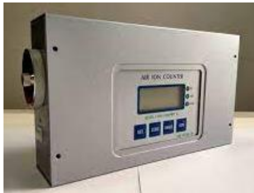
Figure 4: COM 3200 Pro II ion meter used for ion measurements of the PA663 ionizer.
