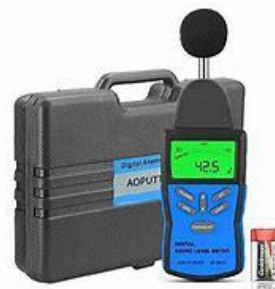
Figure 10. The Aoputriver AP-882A is a digital sound meter with an accuracy of ±1.5 dB with sampling 2 times every second.
