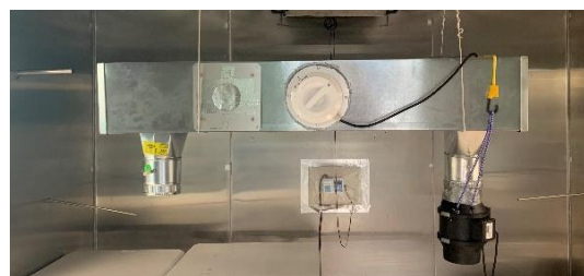
Figure 2: CASPR Medik – Installed in partial HVAC duct used for testing in the bioaerosol test chamber.
