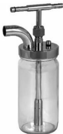
Figure 6. 6-Jet Collison nebulizer. Glass and 304 stainless steel construction, made by BGI Industries.
