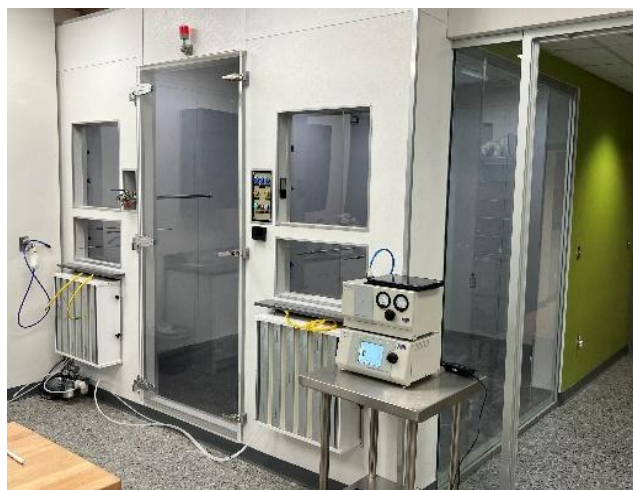
Figure 4: The 30 m 3 bioaerosol testing chamber at ARE Labs adheres to AHAM AC-5 standards and ASHRAE 241 criteria. The chamber is equipped with HEPA filtered air in/out, multiple bio aerosol sampling ports, decontamination, and pressure balance.
