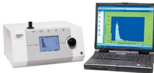
Figure 11. TSI Aerodynamic Particle Sizer (APS) model 3321 used to measure total particle concentration and particle size distribution of the challenge bioaerosol. It has a range of 0.54\text{--}20.0\text{ }\mu\text{m} aerodynamic diameter, with 1 particle/L detection limits.
