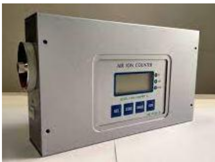
Figure 10: COM 3200Pro II ion meter used for ion measurements of the PA663 ionizer.
